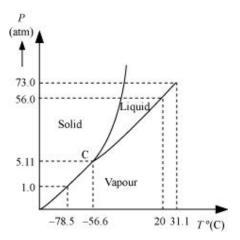
At 1 atm pressure and at -60°C, CO<sub>2</sub> lies to the left of -56.6°C (triple point C). Hence, it lies in the region of vaporous and solid phases.
