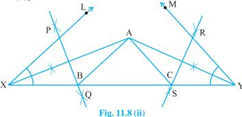
Then ABC is the required triangle. For the justification of the construction, you observe that, B lies on the perpendicular bisector PQ of AX.
