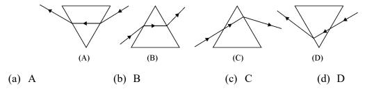
Select the diagram in which the path of a ray passing through a glass prism is correctly drawn
